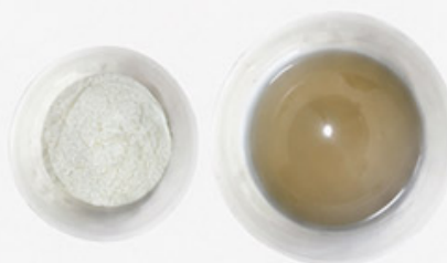
Microsilica + Epoxy Resin + Curing Agent
